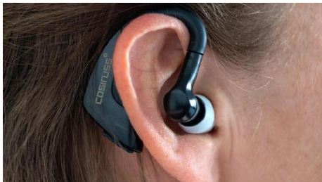
Fig. 13 In-ear sensors Source: Andreas Heddergott / TUM
