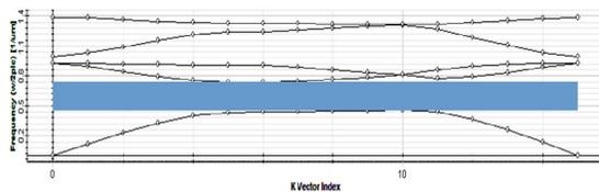
Fig 3: TE band diagram square lattice with defects
