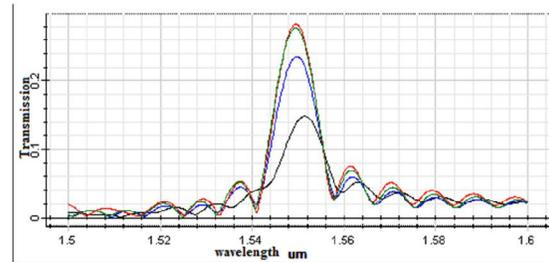
Fig 5: Output transmission spectrum of nanocavity based biosensor
