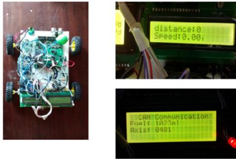
Figure 6.1: (a) Prototype of vehicle (b) Displays the monitoring parameters
