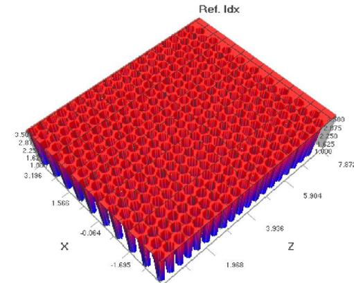
Figure 2. PC structure with ‘air holes in slab’.
