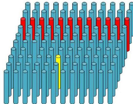
Figure 1. 2D PhC waveguide based on Point defect and Line defect[6].
