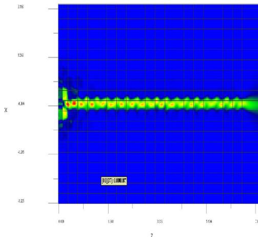
Figure 6. The Magnetic field distribution of the waveguide.
