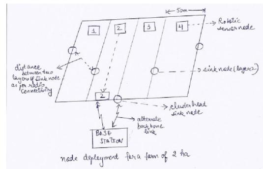
Fig. 2: node deployment for a 2 ha sized farm
