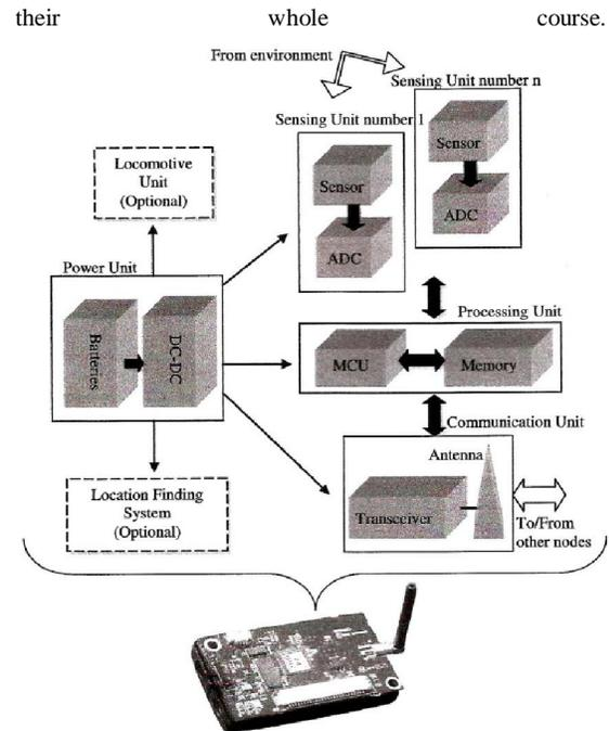
Fig. 1: shows the sensor node hardware.
