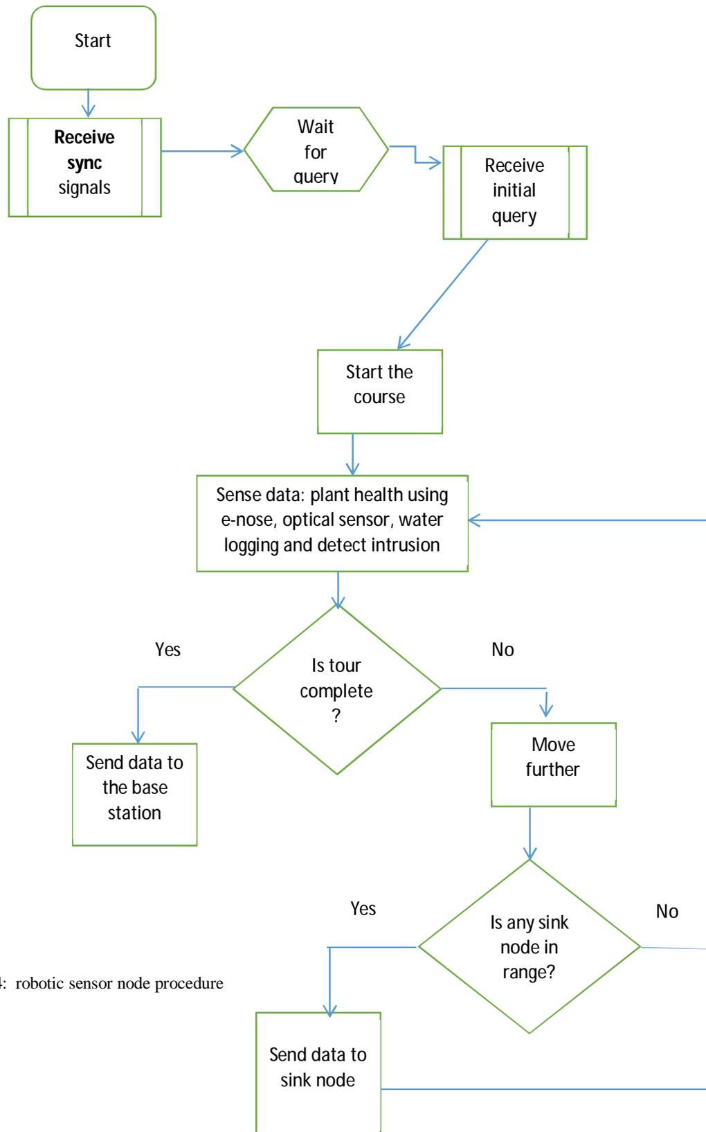
Fig. 4: robotic sensor node procedure
